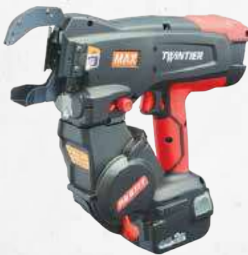
RB611T TIES #5 x #5 UP TO #9 x #10 With 19Ga. Wire
