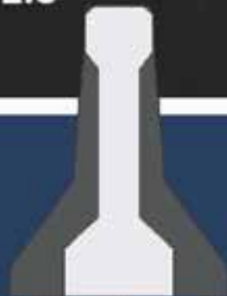
11.75" ZoneBloc+® width VS 24" Jersey barrier width
